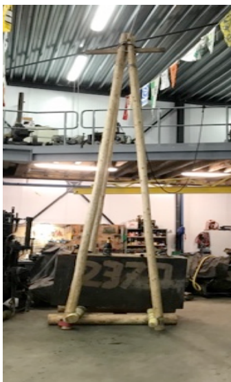
Fig. 3-4. A working tilt levering cage in reality (left) and a detail of the inserted cross bar at the top (right).
