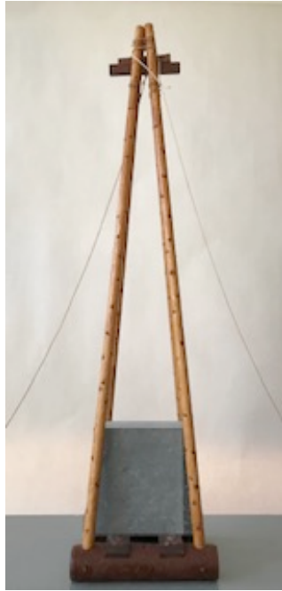
Fig. 5. A working model of a loaded tilt levering cage, Scale 1:10.
