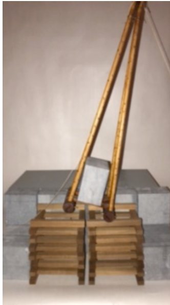
Fig 8. Tilting the model of the tilt levering cage and propping it through box cribbing forming two square stable hollow pillars.
