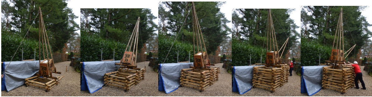
Fig. 3. The author lifted 300 kg using box cribs with a pulling force of about 20 kg and moved this weight horizontally using roller posts with ease. On the right, one additional bipod has been added for tilting by pulling down, click here .
